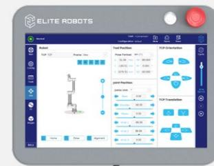
The CS teach pendant contains Elite Robots proprietary software. The optional ERP400S version integrates jogging and function keys and a 3-mode enable key for enhanced safety.
